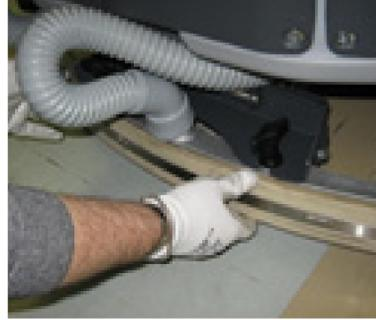
4. Connect the vacuum hose to the squeegee and then fasten it to its assembly
