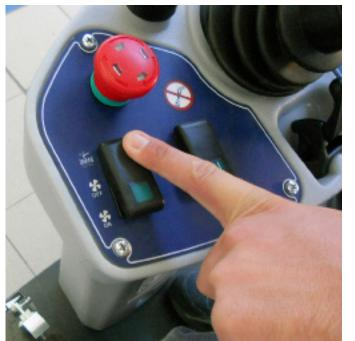
1. Check if all flaps is correctly adjusted 2. Check if the vacuum system switch is 3. Clean the panel filter by pressing the 4. Check if the hopper is full. filter shaker switch.
