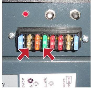
5. Check if the filter shaker fuse (F2) or the vacuum system fuse (F4) is not blown up.
