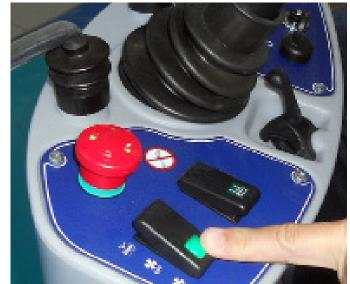
9. Turn on the vacuum system by pushing the switch backward.
