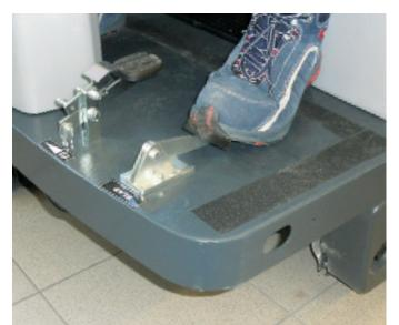
10. To collect light and bulky waste materials, lift the front skirt by pressing the left pedal.
