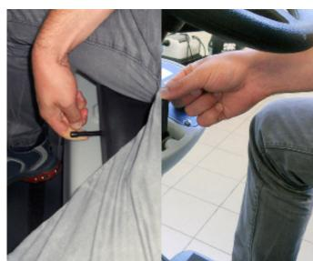
4. Adjust the seat by using the lever. Use the lever to tilt the steering column to a comfortable position.
