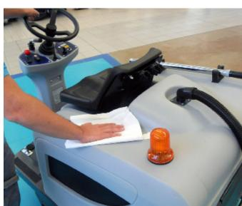
17. Clean the machine by using a damp cloth and where needed use a neutral cleaning product.
