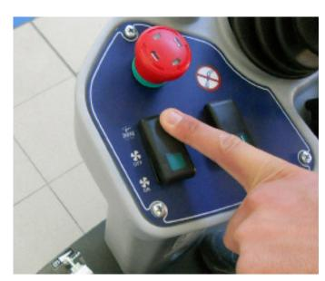
11. To clean the filter, turn on the filter 12. Stop the machine by press the shaker by pressing the switch forward for a few seconds.
