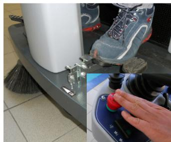
service brake pedal. Press the emergency push-button in case of emergency and to immediately stop the machine functions.
