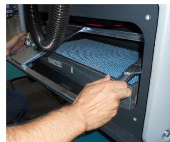
15. WEEKLY: Access to the filter compartment. Remove and clean the dust filter as indicated into the manual.
