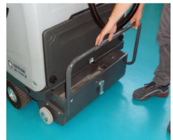
14. Remove the hopper by using the handle and by disengaging it from the inner guides. Discharge all the debris into special containers.
