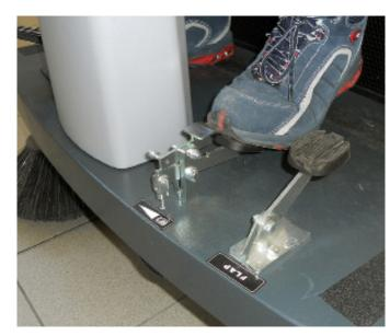
6. Disengage the parking brake by pressing the service brake pedal.
