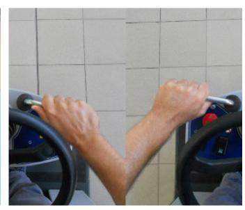
8. Lower the main broom with the right lever; it will start turning. Lower the side brooms with the left lever.
