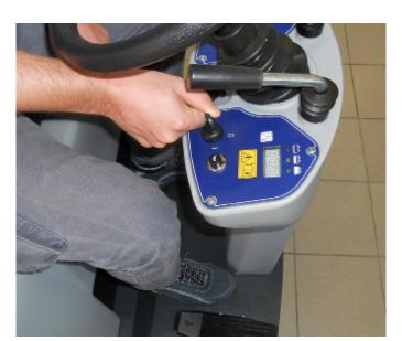
5. Turn the ignition key to "I" and do not press the pedal.
