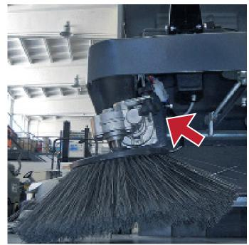
3. Adjust the side broom position by the register knob. Replace the side broom if bristles are worn out.
