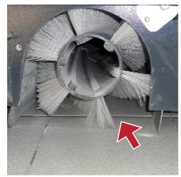
2. Access to the main broom compartment. Check or replace the broom if bristles are worn out.
