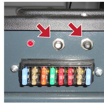
4. Check if the main broom circuit breaker (FA) or the side brooms circuit breaker (FB) is not open.
