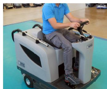
7. Drive the machine by keeping the hands on the steering wheel and pressing the pedal on the front side to move forward and on the rear side to move backward.
