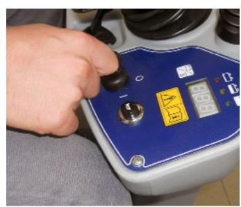
13. Turn off the machine by turn the ignition key to "0".
