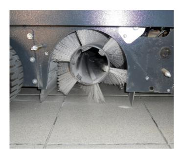
16. WEEKLY: Check the main and side brooms and remove any debris like straps, rope etc.
